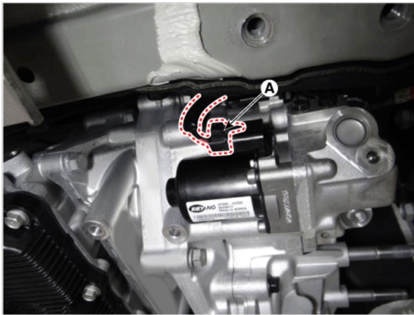
9. Disconnect the pressure sensor connector (A).
