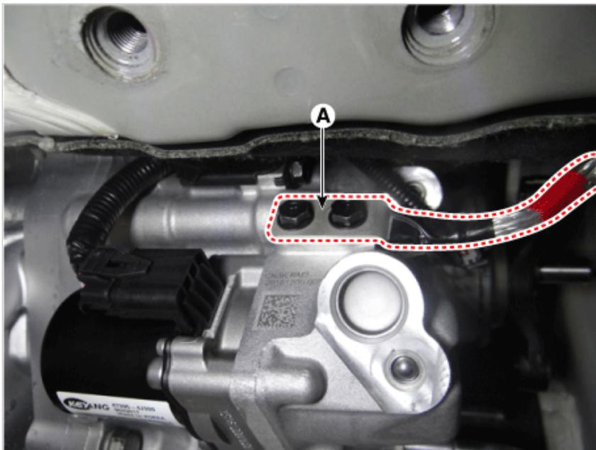
11. Remove the transfer wire ring (A).
